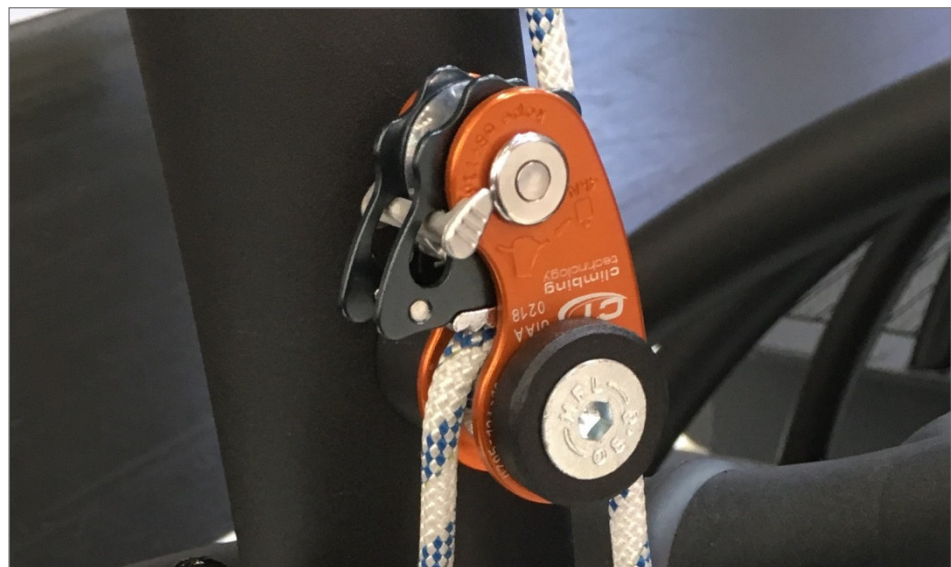
Fig. 8 Rope lock, Locking Pawl Locked
