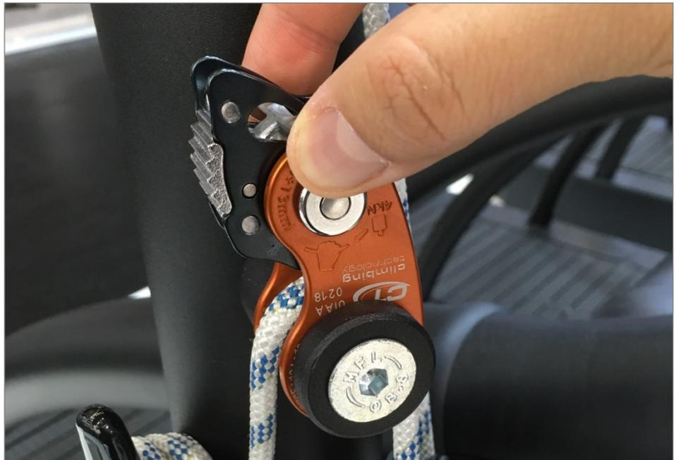
*Fig. 9 Rope lock, Locking Pawl Open*
