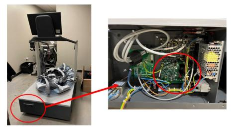
Ensure the Boost 2 is powered down. To remove the fuses, pry them out of the fuse holders with a screwdriver. When replacing, ensure you have glass fuses, 8A 250VAC 5X20MM (littlefuse 0218008.mxp). Insert the fuses back into the fuse holders by inserting one side, and then applying pressure to the other side until they click into place.
