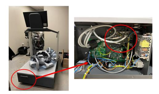
Ensure the Boost 2 is powered down. To remove the fuses, remove the plastic fuse covers and pry them out of the fuse holders with a screwdriver. When replacing, ensure you have glass fuses, 4A 250V AC DC 5mm x 20mm (Bel Fuse PN 5ST 4-R). Insert the fuses back into the fuse holders by inserting one side, and then applying pressure to the other side until they click into place. Finally, replace the plastic fuse covers.
