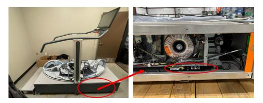
Ensure Boost 2 is powered down. To remove the fuses, push in and make a quarter turn to the left, then remove pressure and they will release. When replacing, ensure you have 250VAC SB Type B, 16A fuses and place them into the fuse holder. Insert the fuse holder into the AC bracket by pushing it in, then applying pressure while turning clockwise until they are properly seated.
