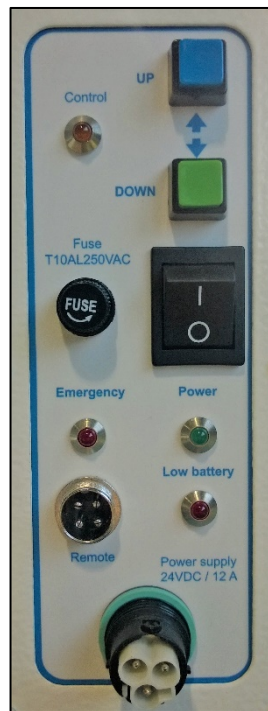
Fig. 17 ELVETA Drive, Control Elements
