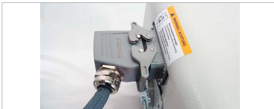
Fig. 39 Checking main plug
