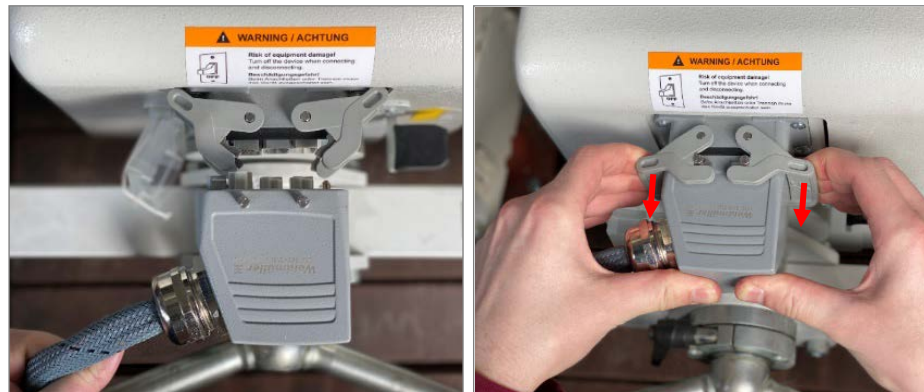
Fig. 11 Connecting and locking control unit connector to the LokoHelp®
