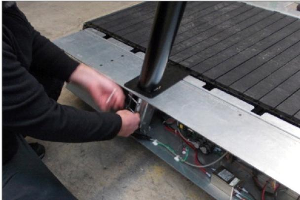
Fig. 31 Pro/ProXL Assembly, Insert Railing
