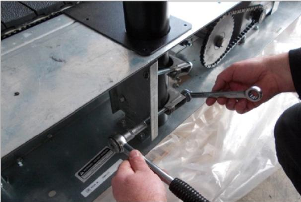
Fig. 38 Pro/ProXL Assembly, Fixing the Railing 2
