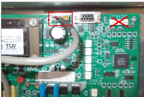
Fig. 26 Mercury/Path Assembly, Connection 4
