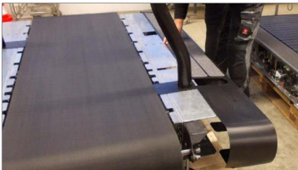
Fig. 7 Removing Side Panel
