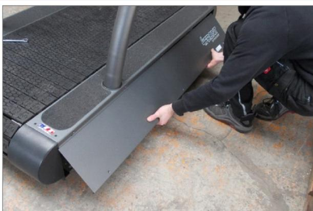
*Fig. 17 4Front Assembly, Side Panel*
