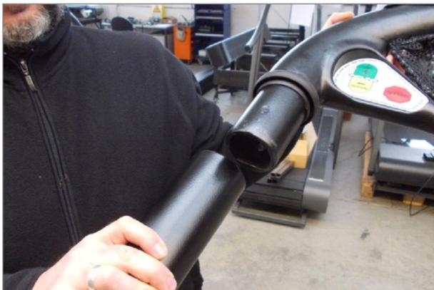
Fig. 32 Pro/ProXL Assembly, Connecting Railing
