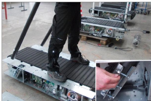
Fig. 22 Mercury/Path Assembly, Insert Tubes
