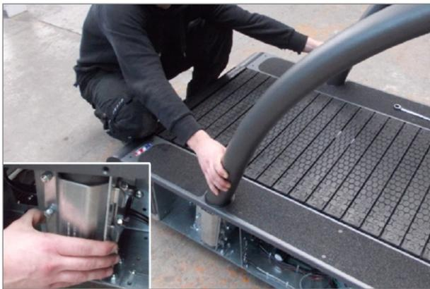
Fig. 12 4Front Assembly, Inserting Tubes
