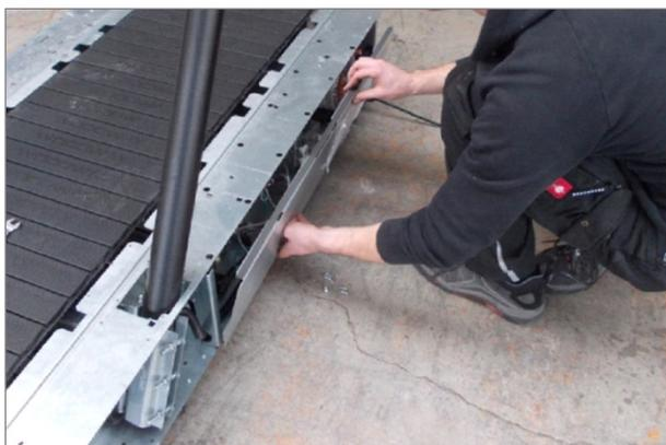
Fig. 28 Mercury/Path Assembly, Electronic Cover Plate
