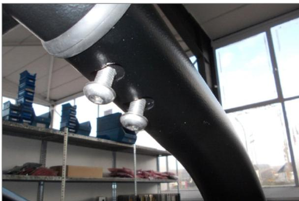
Fig. 33 Pro/ProXL Assembly, Screwing Railing Together
