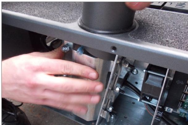
Fig. 11 4Front Assembly, Tube Mount
