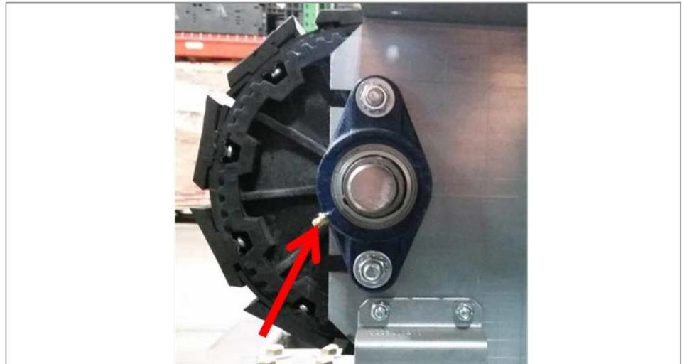
*Fig. 71 Lubrication, Axle bearing*
