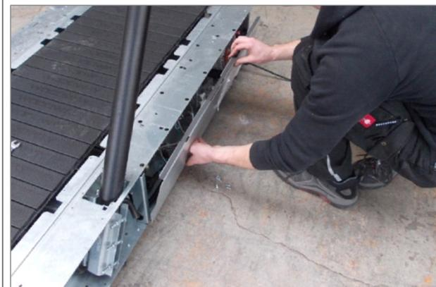
Fig. 19 Mercury/Path Assembly, Electronic Cover Plate
