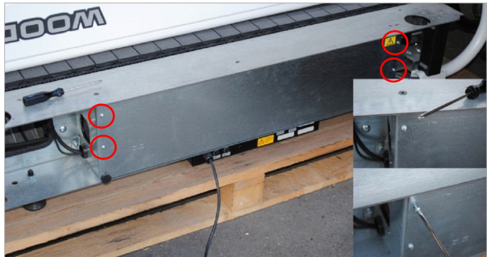
Fig. 6 Remove electronics shielding panel
