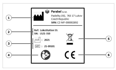
Fig. 3 Nameplate, LokoStation
