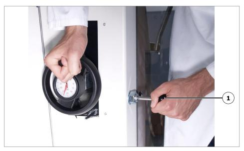
Fig. 11 Locking Pins, Body Weight Support
