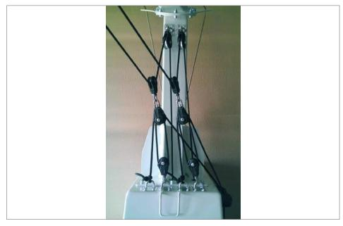
Fig. 23 ELVETA, Two-Sided Rope Length Adjustment
