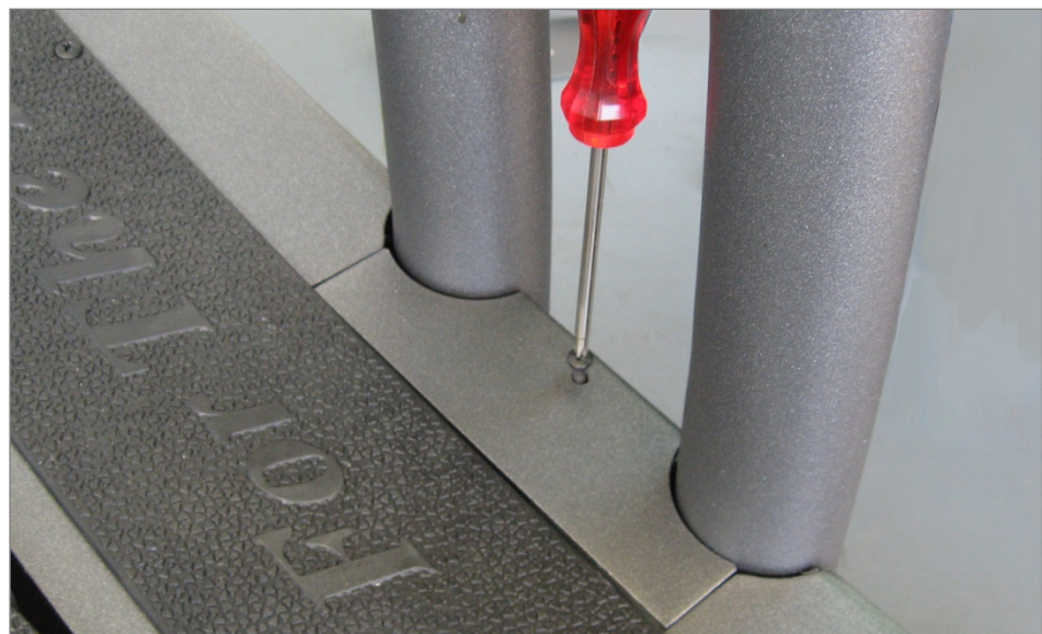
Fig. 17 Installation step, fixing cover plates (CURVE / CURVE XL)
