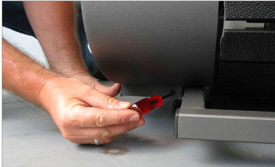
Fig. 8 Installation step, fixing bottom of side panel
