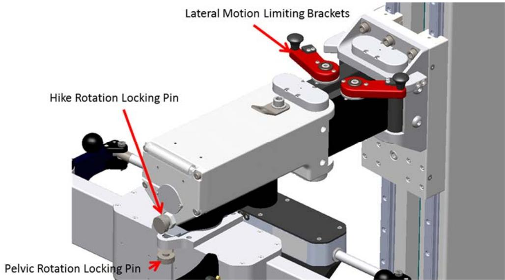
Figure 3 – Passive motion locking mechanisms.
