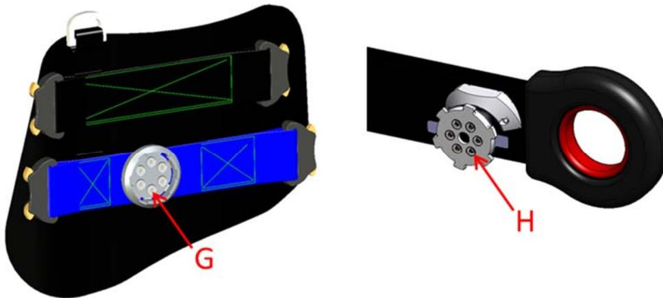
Figure 52 - Illustration showing Pelvic Harness screws
