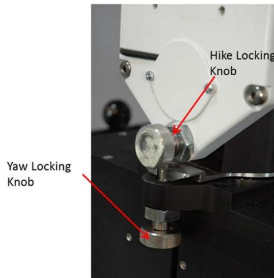
Figure 12 – Locking Knobs
