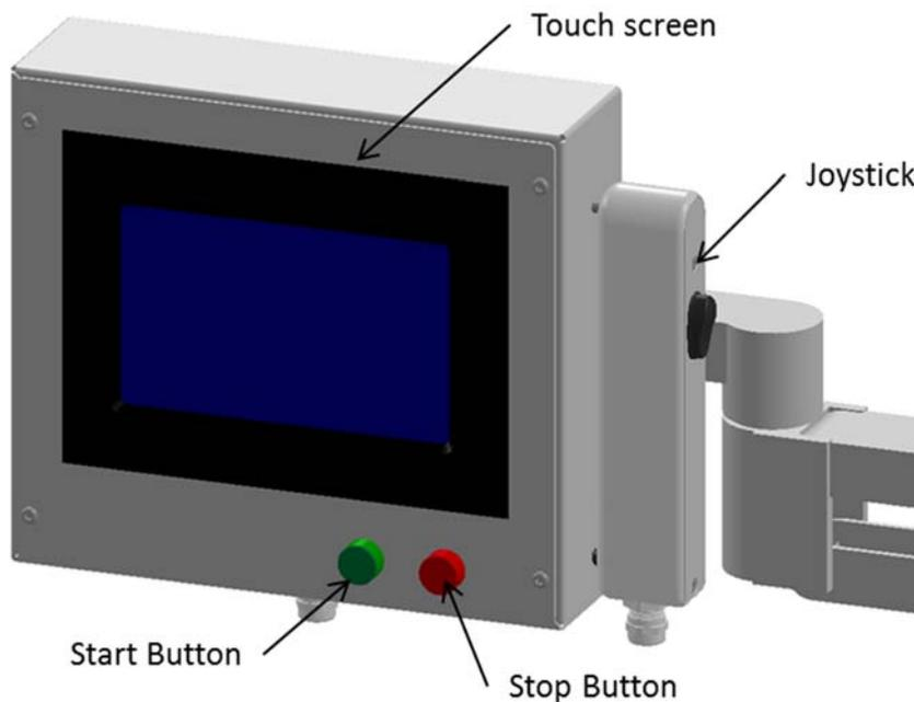
Figure 17 - Illustration of the operator interface.
